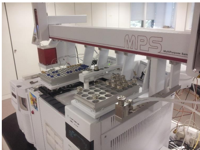
Figure 1: Gerstel Dual Head MPS with flow cell and GC FID
