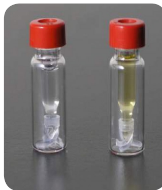
Figure 9: Final oyster SBSE extract (left) compared to dSPE extract (right). Less matrix is co-extracted with SBSE.
