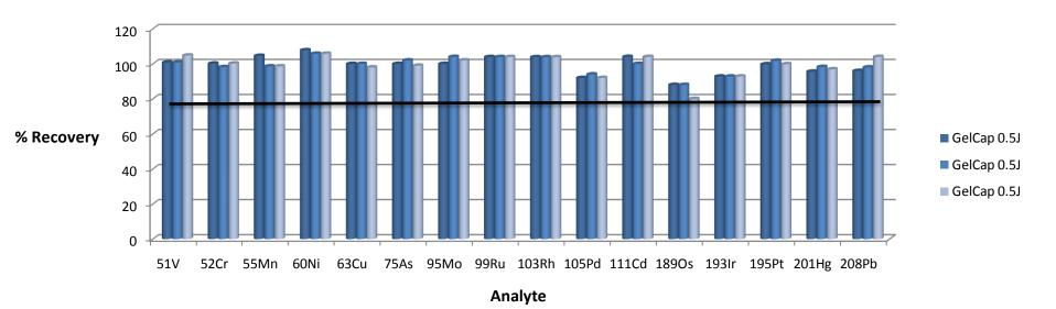
clearly demonstrates that the use of the 7700/7500 ICP-MS with helium mode and KED results in specific, accurate and precise analysis of pharmaceutical samples.
