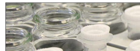
The columns remain sealed on the system - positive pressure ensures constant flow rates.
