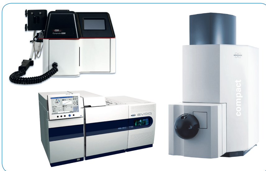
Figure 1: Components of the Pyrolyzer GC APCI QTOF MS system used in this study: (left to right) CDS Analytical Model 6200 Pyroprobe, Bruker Daltonics 456 GC, Bruker Daltonics compact QTOF MS
