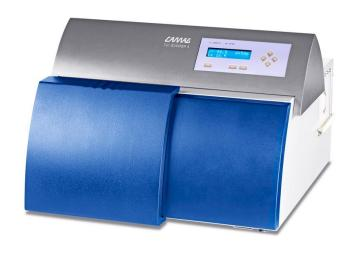
Detection by scanning plates & sheets up to 20x20 cm under specific wavelength in the UV or visible range
