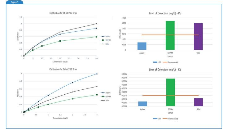
the myth of shorter lifetimes. In terms of performance we see that when the lamp is operated at the recommended current for the multi-element lamp, the sensitivity achieved with the multi-element lamp is comparable to that achieved with a single-element lamp. There may be a slight degradation in the detection limit achieved, but that change is relatively small. Concerns about poor performance of a multi-element lamp is also a myth.
