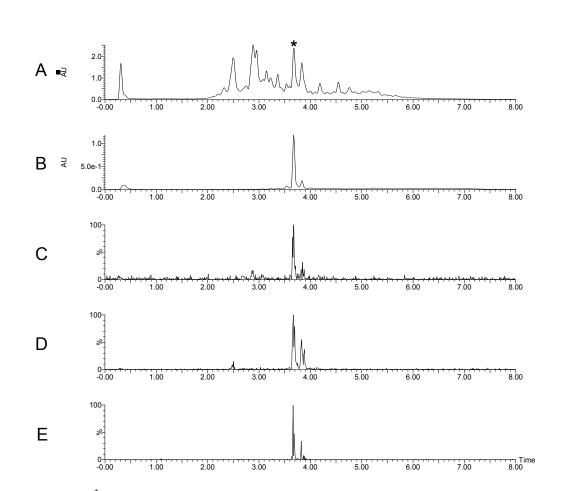
Figure 2. \*Target peak identification in the crude licorice extract, retention time 3.67 min. (A) Total absorbance chromatogram; (B) Glycyrrhizic acid standard, 251 nm; (C)  $[M+H]^{\dagger}m/z = 823.4$ ; (D)  $[M+Na]^{\dagger}m/z =$ 845.4; (E) [M-H]<sup>-</sup> m/z = 821.4; 5-95%B in 5 min; Inj. Vol. 5 μL.
