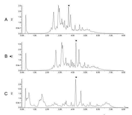
Figure 3. Chromatographic method development for the <sup>\*</sup>target peak in the crude licorice extract; 251 nm; Inj. Vol. 5  $\mu$ L. Mobile phase A = 0.1% FA in water (A) 5-95% B in 5 min; mobile phase B = 0.1% FA in ACN; (B) 5-95% B in 5 min; mobile phase B = 0.1% FA in 3:1 ACN:methanol (C) 25-70%B in 5 min; mobile phase B = 0.1%FA in 3:1 ACN:methanol.
