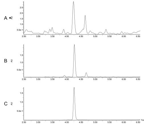
Figure 5. Glycyrrhizic acid identification after isolation. (A) Crude licorice extract, Inj. Vol. 5  $\mu$ L; (B) Glycyrrhizic acid standard, Inj. Vol. 5  $\mu$ L; (C) Peak 1 isolate, Inj. Vol. 10 µL; 251 nm.
