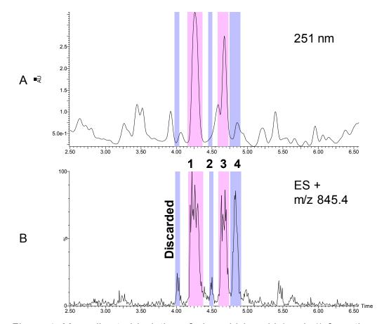
Figure 4. Mass-directed isolation of glycyrrhizic acid (peak 1) from the crude licorice extract; Inj. Vol. 10 µL. (A) UV chromatogram at 251 nm. (B) Extracted chromatogram for the  $[M+Na]^+ m/z = 845.4$  ion. 25-70%B in 5 min; Mobile phase A = 0.1% FA in water; mobile phase B = 0.1%FA in 3:1 ACN:methanol.
