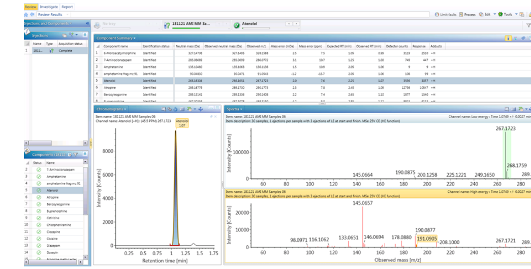
Figure 4. Positive AMI extracted mass chromatogram for atenolol and corresponding MS E precursor/fragment ion MS spectra.
