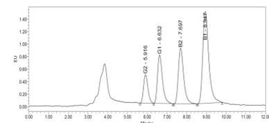
Figure 1: HPLC chromatogram from analysis of a black pepper sample spiked with 4.0 µg/kg total aflatoxin
