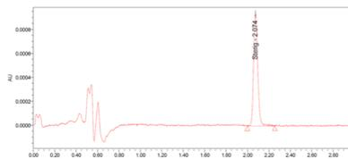
Figure 3: UPLC chromatogram from analysis of corn sample spiked with 25 µg/kg Sterigmatocystin
