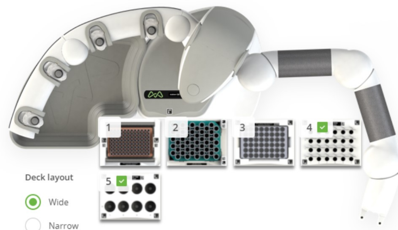
Figure 2. Andrew+ deck configuration for the "Carnitine by LC-MS/MS" protocol. Domino positions on the Andrew+ working deck: [1] Tip Insertion System Domino, [2] 5mL Tip Rack Holder Domino, [3] 2mL HPLC Vial Rack Domino, [4] Microtube Domino, [5] 50mL Conical Centrifuge Tube Domino.
