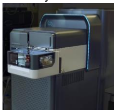
Figure 1. DESI™-XS source with Cyclic IMS.
