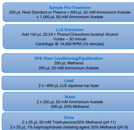
Figure 1. Sample pretreatment and LLE-SPE oligonucleotide extraction protocol using phenol:chloroform and Oasis WAX \mu Elution SPE in the 96-well format, effectively disrupts protein binding ensures high oligonucleotide recovery, aids in selectivity and facilitates sample concentration.
