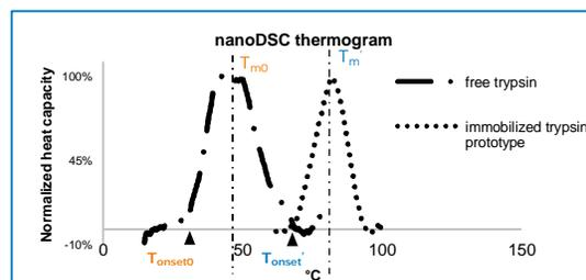
**Figure 1.** NanoDSC thermograms of free trypsin and one optimal immobilized enzyme prototype.  $T_m$  – temperature where half of the protein is unfolded;  $T_{onset}$  – temperature where protein starts to unfold.
