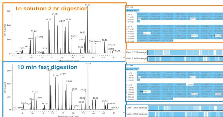
**Figure 2.** The peptide mapping results comparing the 2 hr trypsin digestion workflow vs. the 10 min fast digestion workflow. Left panel: LC-MS chromatogram; Right panel: sequence coverage of light chain and heavy chain respectively.
