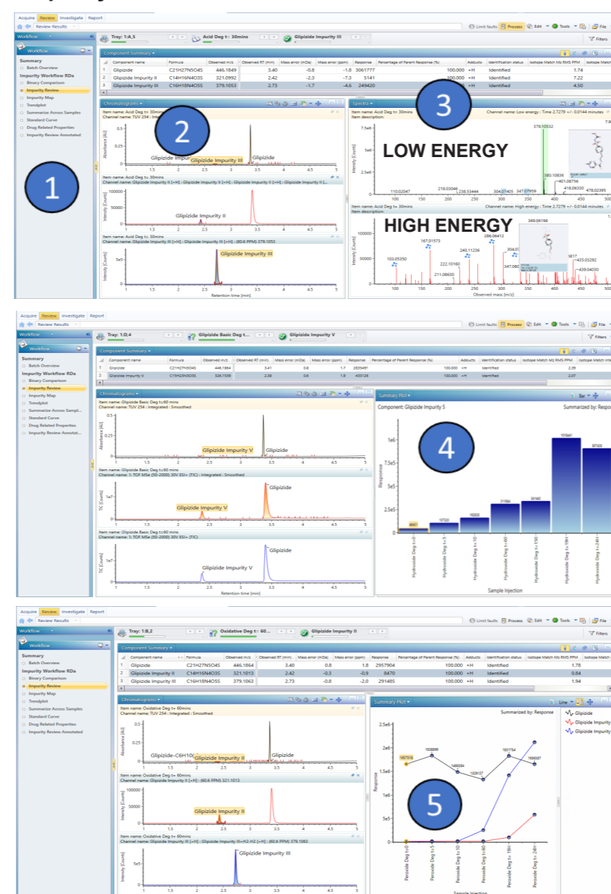
Figure 3. Top: Acid degraded glipizide with 'impurity profile' selected in the workflow (1), main review pane (2) showing UV and XIC of impurity II and III. Impurity III is selected showing high and low energy acquisitions (4) with structural visualisation of the impurity and an associated fragment. Middle: Basic degradation with increase of impurity V plotted in the summary plot (4). Bottom: Oxidative degradation with line graph overlay of glipizide and concomitant generation of impurities II and III over time.
