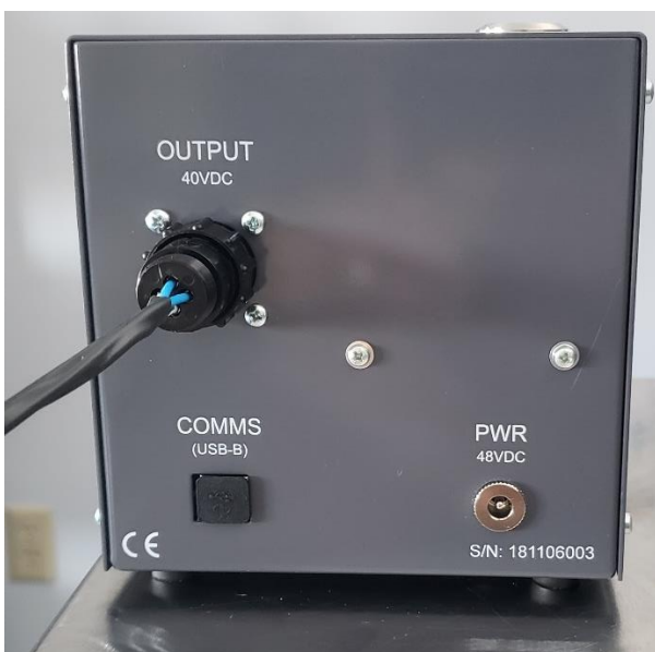
Figure 5. (B). ARC Temperature Controller box with adapter cable connected to the 40VDC “Output”.
