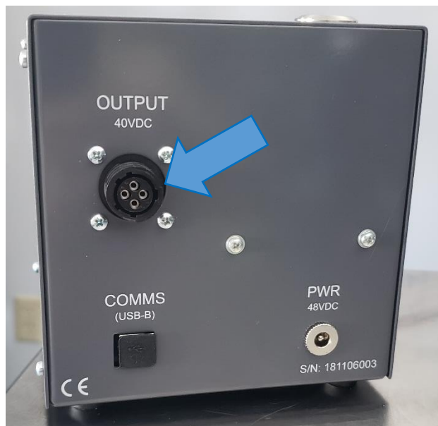
Figure 5. (A). Locating 40VDC “Output” on back of ARC Temperature Controller box.
