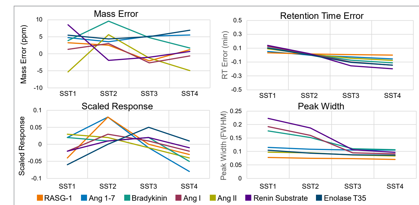
Figure 4. System suitability injections of a peptide standard mixture on a BioAccord System were used at the beginning and end of the MAM analysis sample sequence to ensure the system was producing results within established performance specifications. These injections are flagged in the Peptide MAM App's sample list and evaluated on specified criteria, including mass error, retention time error, scaled response, and peak width. Shown here are the trends summarized in the Peptide MAM App as part of the BioAccord LC-MS MAM workflow.
