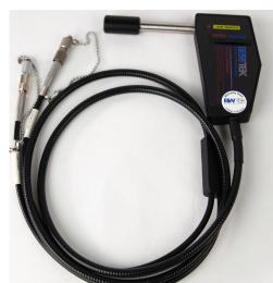
The BAC100B series Raman probe is a versatile sampling interface for use with our portable Raman instruments. It is identical to the BAC102 series except without the trigger. The probe can be brought directly to the sample and make contact with either the sample or the packaging of the sample via a detachable distance regulator that ensures proper focusing while minimizing contamination to the lens material.
