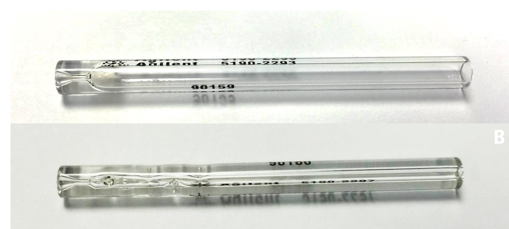
Figure 3. Typical GC inlet liners appearance after 100 injections of avocado samples prepared by EMR-Lipid cleanup followed with enhanced post treatment. A) UI single taper splitless liner with wool, B) UI dimple liner.
