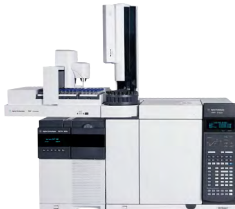
Agilent GC 7890 GC equipped with an FID and 5977 MSD.
