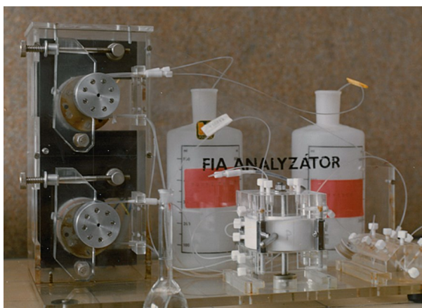
Fig. 1. The FIA analyzer constructed at the Department of Analytical Chemistry, Faculty of Pharmacy in Hradec Králové, Charles University. Manufactured in cooperation with the Unified Agricultural Cooperative “1 st of May” in the village of Pouchov near Hradec Králové (the 1980s). Multi-channel analyzer equipped with two peristaltic pumps, double injection valve, and unit with mixing points. For optical detection, used Spekol photometer with a flow cell.
