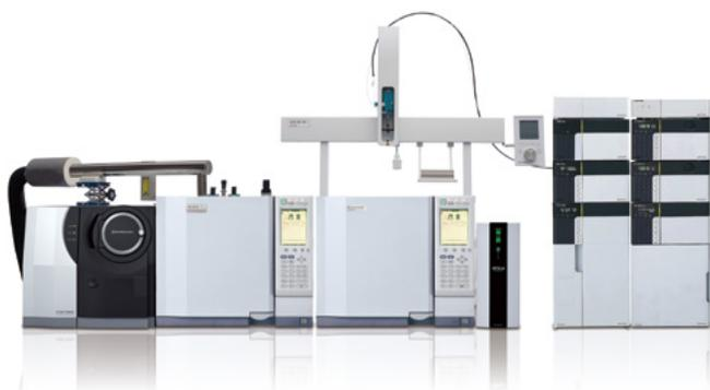
Fig. 1 LC-GC×GC-MS/MS instrumentation
