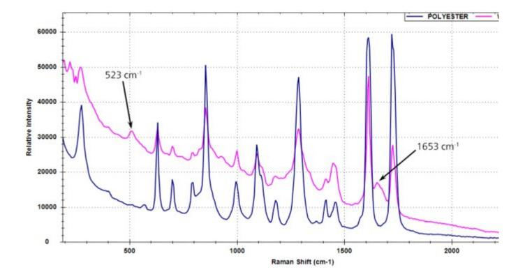
Figure 2. Overlay of spectra for wool and polyester
