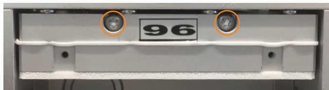
Figure 5. The two screws attaching the pressure head to the pressure unit.
