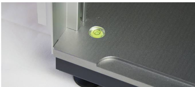
Figure 3. The built-in spirit level in the bottom of the system, in the front left corner.
