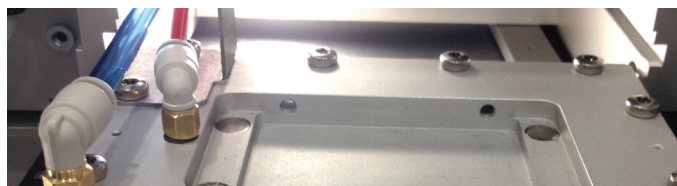
Figure 6. System with two gas tubes connected to the pressure head.
