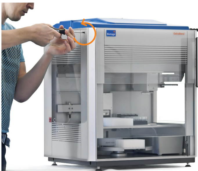
Figure 15. Open the door manually by turning the screw counterclockwise.
