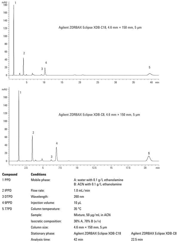
Figure 1. Column stationary phase comparison for five PPDs.
