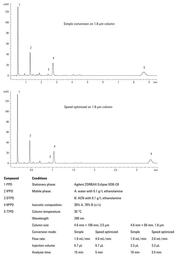
Figure 2. Separation of five PPDs on a smaller particle size column using the transferred methods.
