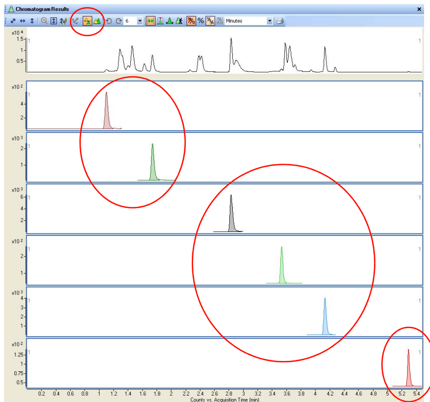
Figure 4 Extracted chromatograms in Qualitative Analysis Chromatogram Results window. The List Mode icon is circled in the toolbar of the Chromatogram Results window shown here.
