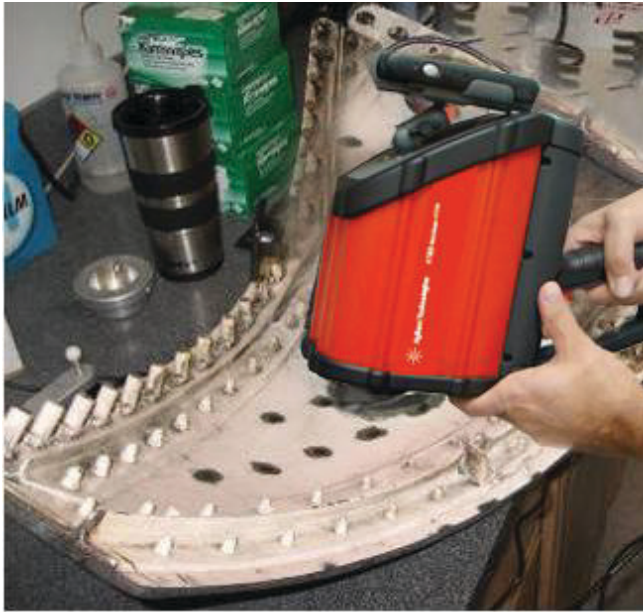
Figure 5. A 4100 ExoScan FTIR being used to measure heat damage on a composite aircraft part, which had been damaged by an engine fire
