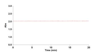
Figure 2. Continuous kinetics absorbance readings measured every 12.5 ms, of methylene blue (20 ppm) at 664 nm
