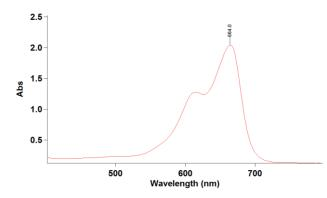
**Figure 1**. Ten superimposed wavelength scans of methylene blue (20 ppm) solution in water. As can be seen, the scans overlay perfectly confirming the accuracy of the Cary 60 UV-Vis and the absence of any photobleaching of the sample
