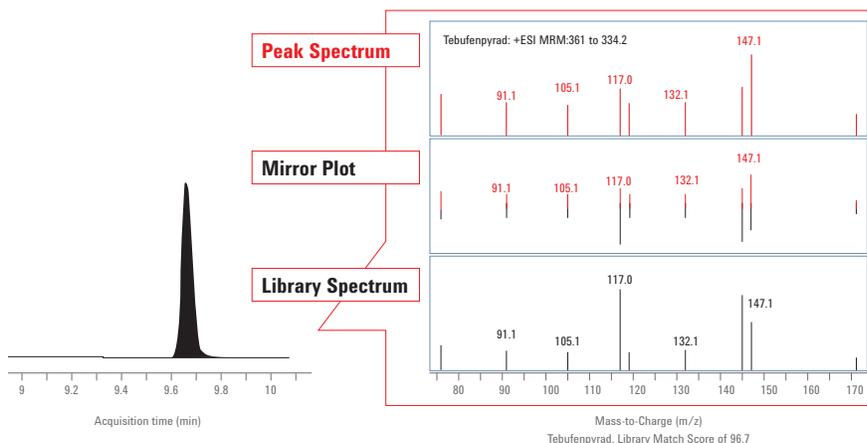
The above figure, generated with data gathered using an Agilent 6460 Triple Quadrupole, shows how the acquired mass spectrum (upper window) can be compared to a stored library spectrum (bottom window). The mirror plot in the central window simplifies the comparison between the sample and library spectra. An excellent library match score of 96.75 confirms the identity of the compound.
