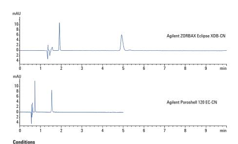
Columns: Agilent Poroshell 120 EC-CN,  $3.0 \times 100$  mm,  $2.7 \mu m$  (p/n 695975-305)
