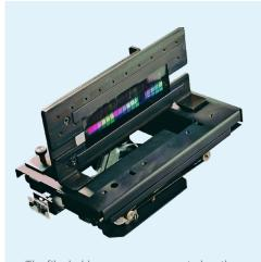
The film holder accessory, mounted on the sample transport accessory
