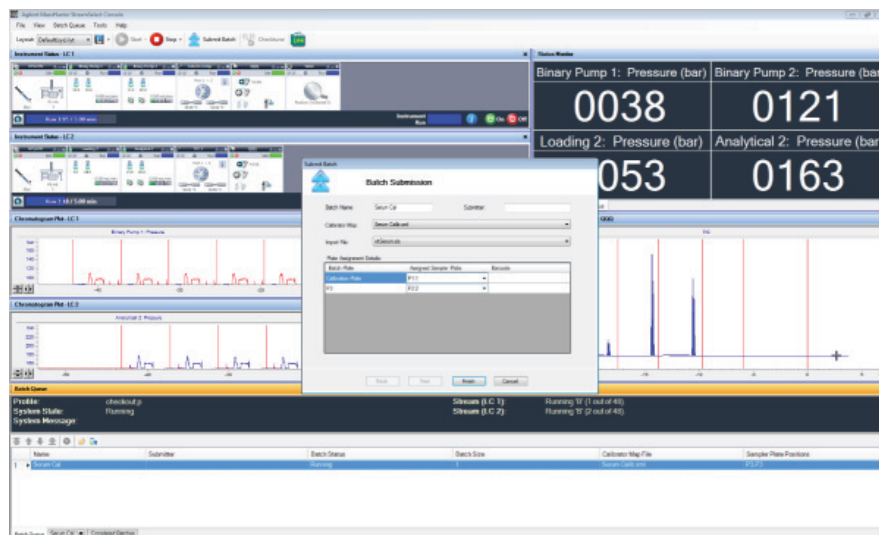
Figure 5. The user Interface of the Agilent MassHunter StreamSelect Software enables three-click batch submission and easy system monitoring.
