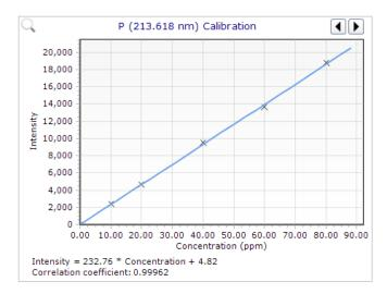
Figure 1. Calibration curve for phosphorus
