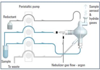
Figure 1. The Multimode Sample Introduction System (MSIS) operation
