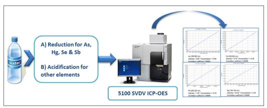
Figure 2. Schematic of water analysis workflow using the Agilent 5110 ICP-0ES
