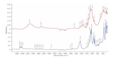
**Figure 8.** Overlaid FTIR spectra of the paper backing from cold medicine blister packs collected using an Agilent Cary 630 FTIR with diamond ATR module. Red: microcrystalline cellulose. Blue: styrene-acrylate copolymer. Most blister packs use the microcrystalline cellulose backing (red), however, one name brand product used the styrene-acrylate copolymer material (blue), which contains very strong bands for calcium carbonate and kaolin clay.
