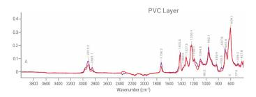
**Figure 3.** FTIR spectra of clear blister polymers from over-the-counter cold medicines collected on a Cary 630 FTIR with diamond ATR module. The outer blister layer of a generic product (red) is overlaid with the inner blister layer of a brand name product (purple). The band at 1736 cm<sup>-1</sup> indicates the presence of ~2–3 % of a copolymer such a polyacrylate or polyvinylacetate.
