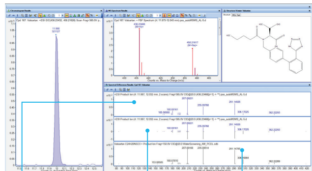
Top: Auto MS/MS spectrum Middle: Mirror spectrum Bottom: Library spectrum
