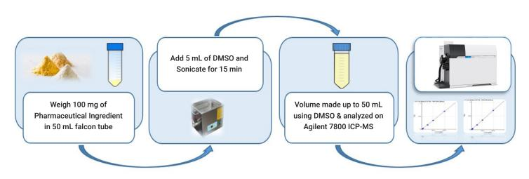
Figure 1. Flow diagram for sample preparation and analysis using the Agilent ICP-MS.
