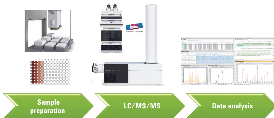
Figure 1. Integrated workflow for peptide mapping mAbs, from automated sample preparation on the Agilent AssayMAP Bravo Platform to Agilent 6550 Q-TOF LC/MS/MS analysis, and Agilent BioConfirm B.08.
