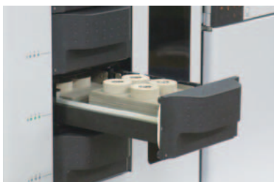
Rack changer: max. 48 samples
