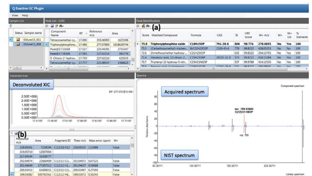
Figure 5. Identification of peak at 17.49 minutes as triphenylphosphine oxide. Screenshot of the deconvoluted data and library match in TraceFinder. (a) List of library hits sorted by score (combination of SI and HRF). (b) List of fragment ions from EI spectrum and elemental composition based on elements in top hit.
