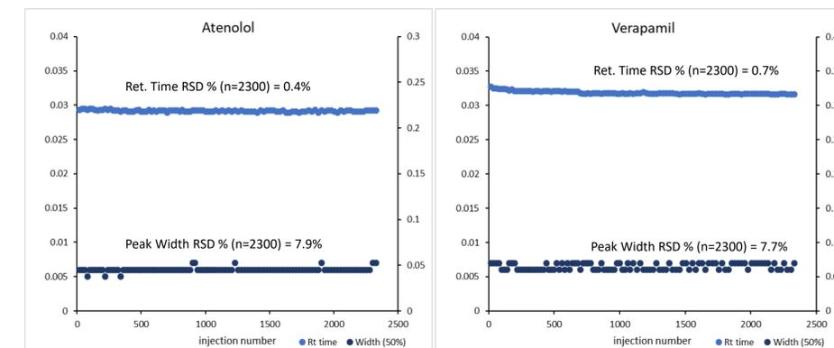
Figure 5 Retention time and peak width for the first eluting molecule over 2300 injections range.
