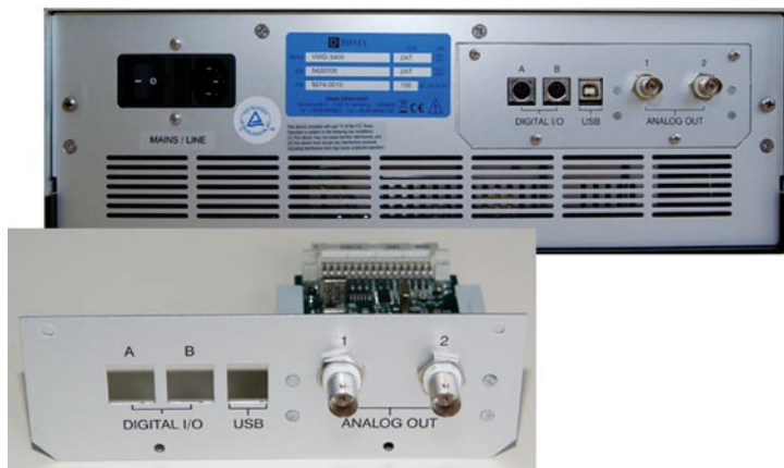
Figure 10. Using standard tools, the optional D/A converter can be installed at the instrument's rear panel in just a few minutes.
