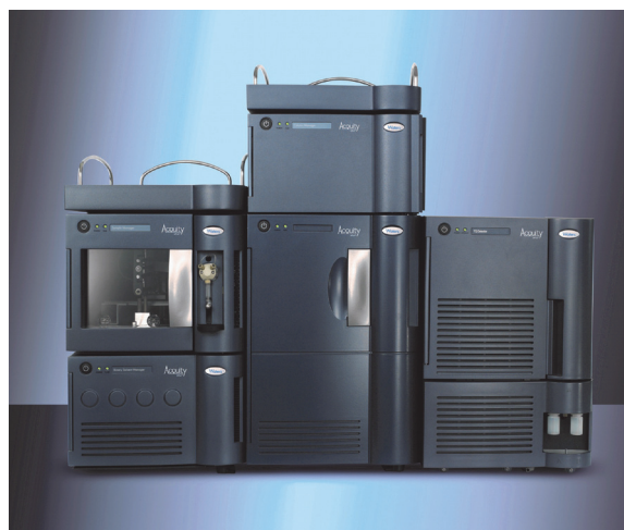
Figure 1. System configuration of a Waters ACQUITY UPLC coupled to a MassTrak Online SPE Analyzer and ACQUITY TQ Detector.
