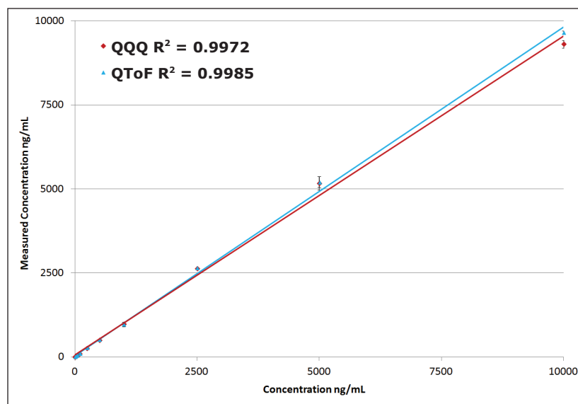
Figure 1. Standard curve comparison by platform: QTof versus tandem quadrupole MS (QQQ), and measured versus reported concentrations.
