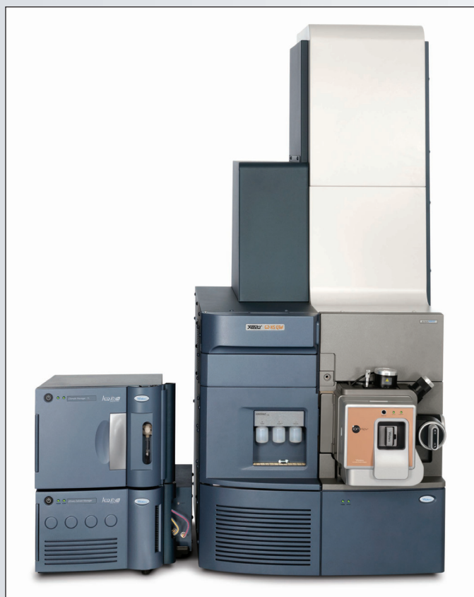
Figure 2. ionKey/MS system with ACQUITY UPLC M-Class System and Xevo G2-XS QTof.
