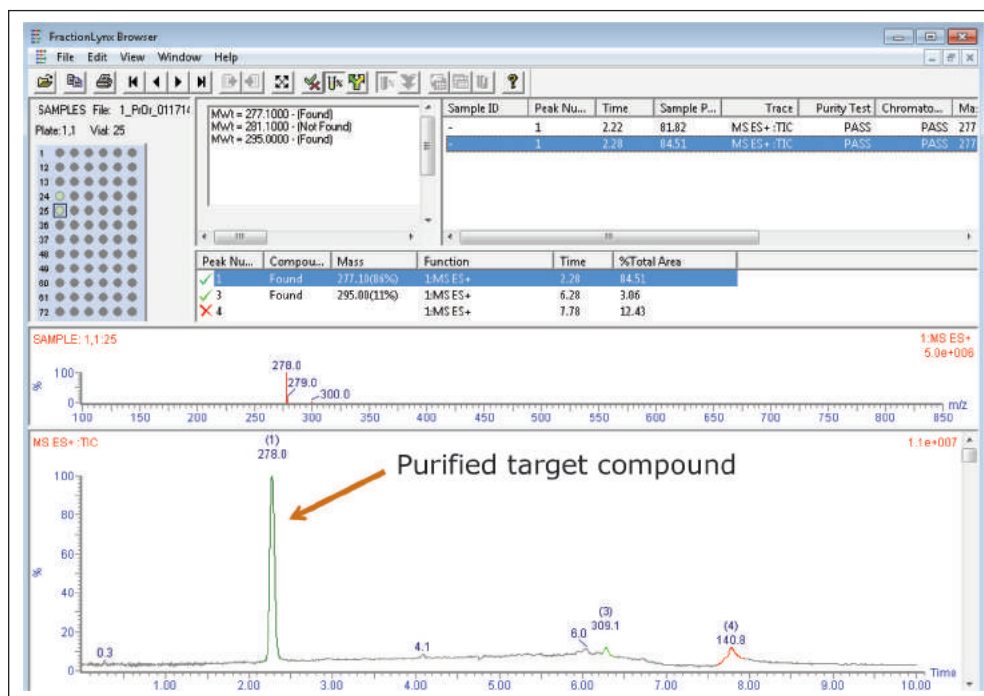
Figure 4. Browser report for the analysis of a fraction. The injection volume was 20 \mu L, taken directly from the collection tube immediately after purification.
