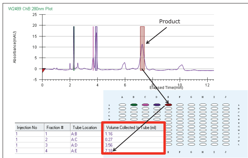
Figure 4. Fraction tracking shows the product tube location in the collection bed as well as the volume collected in each tube.
