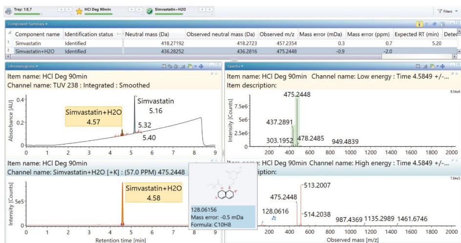
Figure 6. UV/XIC of HCl degraded simvastatin with high energy fragment ion highlighted.
