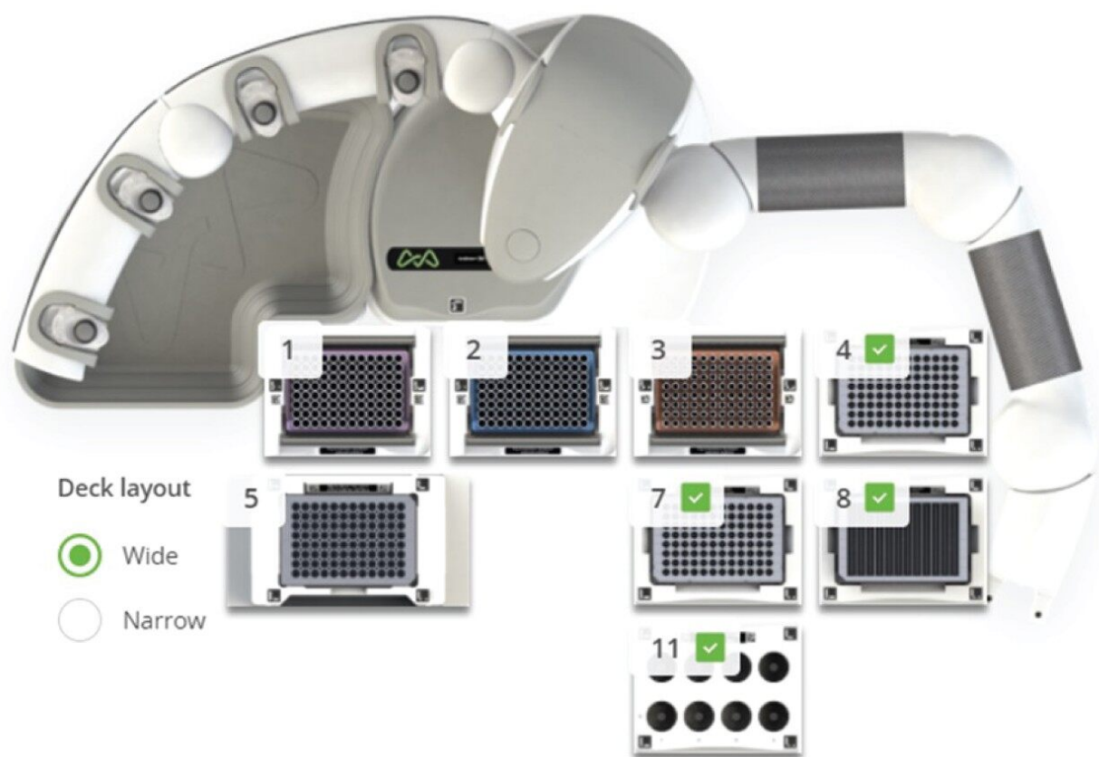
Figure 2. Andrew+ Pipetting Robot workbench layout and configuration for automating the Oasis 2x4 SPE Sorbent Selection Method, as shown in OneLab.
