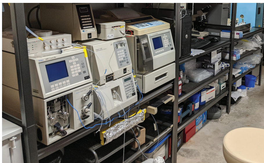
Dr. Register started with a used Waters 600 HPLC System in his garage laboratory, which worked well for this early stage, despite the older analytical technology.
